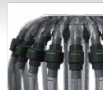
Single electric row shut-off (max. 9+9 motors)
