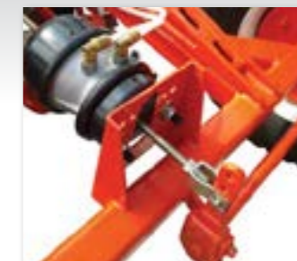
Pneumatically controlled braking system
